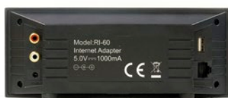
RCA connection to amplifier
